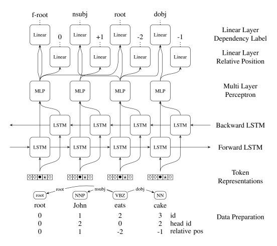
Figure 1: PaT architecture: we feed a concatenation of several representations (Section 3.1.) to a BiLSTM and then a multilayer perceptron (MLP). The MLP output is passed through a linear layer to predict the relative positions. Once a head has been selected, we concatenate the MLP output for the dependent and the predicted head, and pass it to another linear layer to predict the corresponding dependency label.
